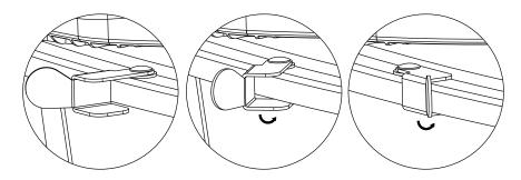
To unlock: lift up on lock handle, remove lock bracket from rise on lid, push lock handle down.
