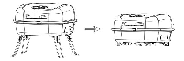
Unfold grill (Note: Always open legs completely and are secured in place before lighting).
