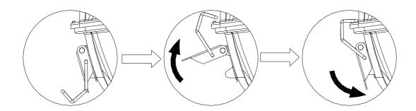
B: Unlock the lid: Lift up on lock handle, remove lock bracket from rise on lid, push lock handle down.
