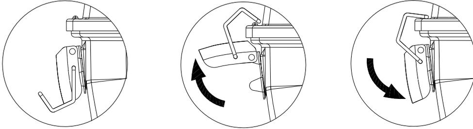
B: Unlock The Lid: Lift up on lock handle, remove lock bracket from rise on lid and push lock handle down.
