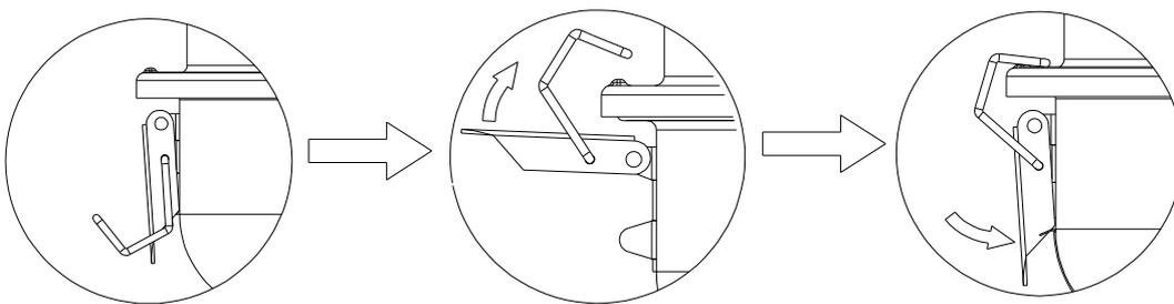
B: Unlock the lid: Lift up on lock handle, remove lock bracket from rise on lid, push lock handle down.
