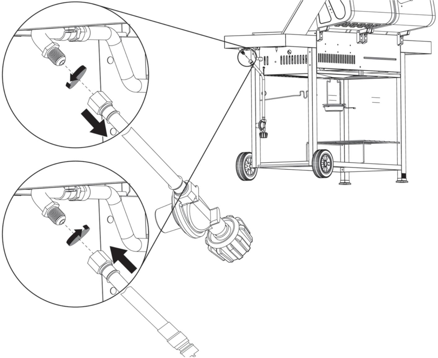
**8 Attach Side Burner Grid, Igniter Wire and Side Burner**
